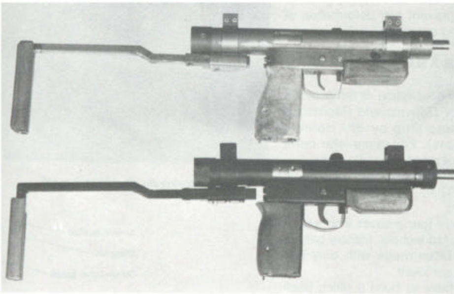
Improvised prototype, including plugs without threading, welded bracket, and plastic pistol grip (top) compared with the standard prototype (bottom).
